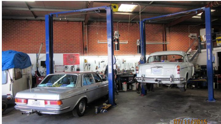
Trevor Page checking the lights, horn, wipers, and indicators as members drove into the workshop. A steady stream of cars all morning from start time at 9.00 am. kept Bob and Anthony busy. Most went up on the hoist for an underbody and mechanical inspection, then a brake test using a modern digital tester.
