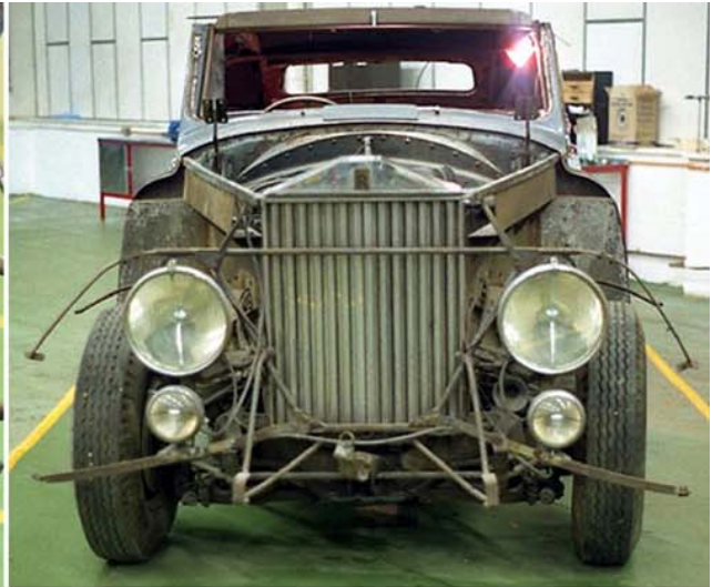
This picture shows the genuine Rolls Royce radiator shell still in place behind the custom front end.
