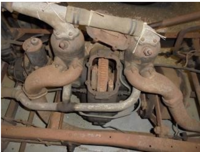
View showing the 2 cylinder two stroke water cooled engine with torque converter inertia weights and engine flywheel in between
