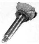
corrosion salts filled the space behind the water pump impeller, to the extent that running the engine had totally ground away the vanes of the impeller. The water pump was now just acting as a baffle, impeding the flow of coolant in what had become a thermosiphon system! And why had we used so much oil? Well, the engine overheating had caused the top lands of the pistons to break down, allowing the two top
